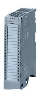
SIPLUS S7-1500 AI 8XU/I HF -40... +70 °C with conformal coating BasedOn: 6ES7531-7NF00-0AB0 . 16 Bits of Resolution, Accuracy 0.1%, 8 Channels in groups of 1; common mode Voltage: 30V AC/60V DC, Diagnosis, Processalarms; incl. infeed element, Shield clamp and Shield terminal
