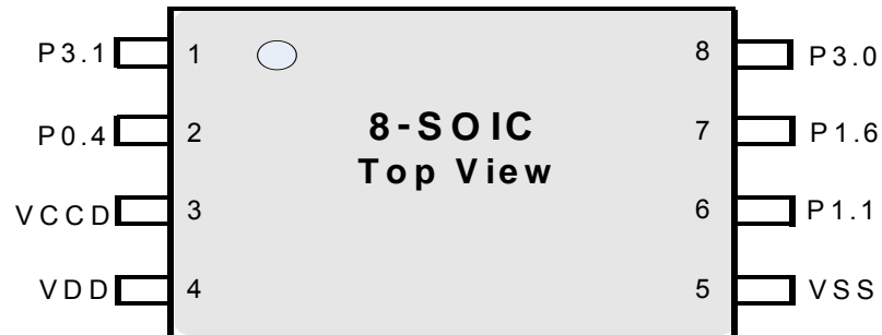
Figure 8. 8-Pin SOIC Pinout
