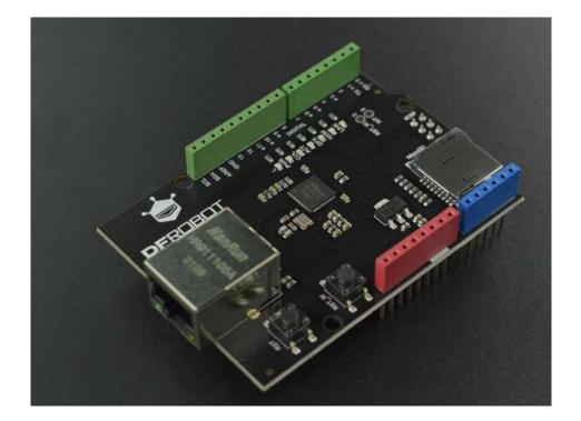
DFRduino Ethernet Shield V3.0 - W5100S (Support Mega and Micro SD)
