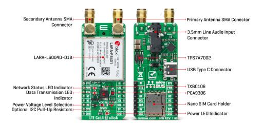
The LTE Cat. 4 3 Click is equipped with a nano SIM card holder for both 1.8V and 3.0V SIM types. The module also includes a USB high-speed 2.0-compliant interface with a minimum 480Mbps data rate. The module itself acts as a USB device and can be connected to any compatible USB host. It provides a virtual serial port over USB for AT commands and communication, a virtual serial port over USB for diagnostic logs, and more.
