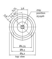
UVC-only SiC based UV photodiode A = 1,0 mm<sup>2</sup>
