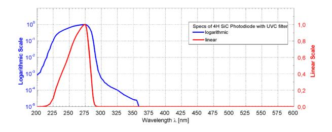
UVC-only SiC based UV photodiode A = 1,0 mm<sup>2</sup>
