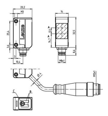
A Optical axis B Indicator diode
