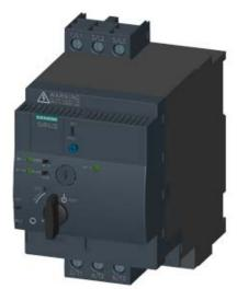
SIRIUS, COMPACT STARTER, REVERSING STARTER 690 V, 24 V AC/DC, 50 ... 60 HZ, 0.32 ... 1.25 A, IP20, MAIN CIRCUIT CONNECTION: SCREW TERMINAL, AUXILIARY CIRCUIT CONNECTION: PLUG-IN, W/O TERMINALS
