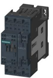
CONTACTOR, AC-3, 18.5KW/400V, 1NO+1NC, DC 24V, 3-POLE, SZ S0 SPRING-LOADED TERMINAL
