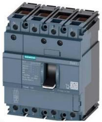
CIRCUIT BREAKER 3VA1 IEC FRAME 100 BREAKING CAPACITY CLASS B ICU=16KA @ 415 V 4-POLE, LINE PROTECTION TM210, FTFM, IN=80A OVERLOAD PROTECTION IR=80A FIXED SHORT CIRCUIT PROTECTION II=10 X IN NEUTRAL UNPROTECTED CABLE CONNECTION
