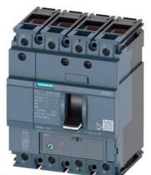
CIRCUIT BREAKER 3VA1 IEC FRAME 160 BREAKING CAPACITY CLASS M ICU=55KA @ 415 V 4-POLE, LINE PROTECTION TM220, ATFM, IN=125A OVERLOAD PROTECTION IR=87,5A ...125A SHORT CIRCUIT PROTECTION II=10 X IN NEUTRAL PROTECTION 100% CABLE CONNECTION
