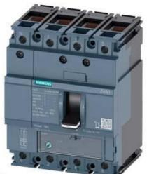
CIRCUIT BREAKER 3VA1 IEC FRAME 160 BREAKING CAPACITY CLASS N ICU=25KA @ 415 V 4-POLE, LINE PROTECTION TM220, ATFM, IN=80A OVERLOAD PROTECTION IR=56A ...80A SHORT CIRCUIT PROTECTION II=10 X IN NEUTRAL PROTECTION 100% CABLE CONNECTION
