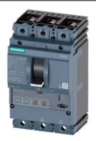
CIRCUIT BREAKER 3VA2 IEC FRAME 100 BREAKING CAPACITY CLASS M ICU=55KA @ 415 V 3POLE, LINE PROTECTION ETU330, LIG, IN=40A OVERLOAD PROTECTION IR=16A ...40A SHORT CIRCUIT PROTECTION II=1,5...12 X IN GROUNDFAULTPROTECTION IG=0,2... 1 X IN, TG=0,1/0,3MS BUSBAR CONNECTION
