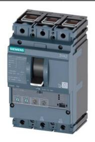
CIRCUIT BREAKER 3VA2 IEC FRAME 160 BREAKING CAPACITY CLASS M ICU=55KA @ 415 V 3POLE, LINE PROTECTION ETU350, LSI, IN=40A OVERLOAD PROTECTION IR=16A ...40A SHORT CIRCUIT PROTECTION ISD=1,5... 10 X IR, II=12 X IN CABLE CONNECTION
