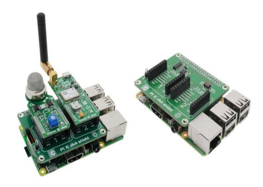
Picture on the right shows Pi 3 click shield connected to the Raspberry Pi $\otimes$  3 model B, picture on the left shows the connected shield along with two click boards $^{\text{TM}}$ : Ozone 2 and GNSS 5 click.
