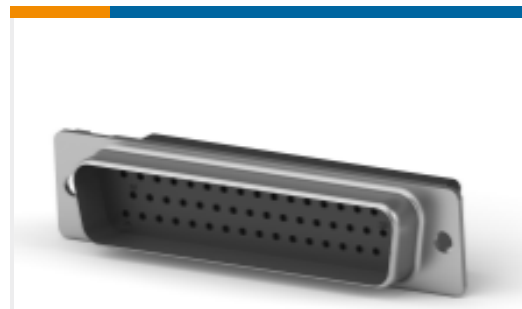
TE Part #1658641-2 D-Sub Crimp: Plug, Signal, 50 Posn, Pin Size 20, Shell Size 5
