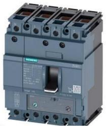
CIRCUIT BREAKER 3VA1 IEC FRAME 160 BREAKING CAPACITY CLASS S ICU=36KA @ 415 V 4-POLE, LINE PROTECTION TM240, ATAM, IN=40A OVERLOAD PROTECTION IR=28A ...40A SHORT CIRCUIT PROTECTION II=5...10 X IN NEUTRAL UNPROTECTED CABLE CONNECTION
