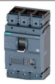
CIRCUIT BREAKER 3VA2 IEC FRAME 630 BREAKING CAPACITY CLASS M ICU=55KA @ 415 V 3-POLE, LINE PROTECTION ETU560, LSIG, IN=400A OVERLOAD PROTECTION IR=160A ...400A SHORT CIRCUIT PROTECTION ISD=0,6..10X IN, II=1,5..15X IN NEUTRAL PROTECTION OPTIONAL WITH EXT. CT;UPTO 160% GROUND-FAULT, SWITCHABLE IG=0,2... 1 X IN, TG=0,05-0,8MS BUSBAR CONNECTION
