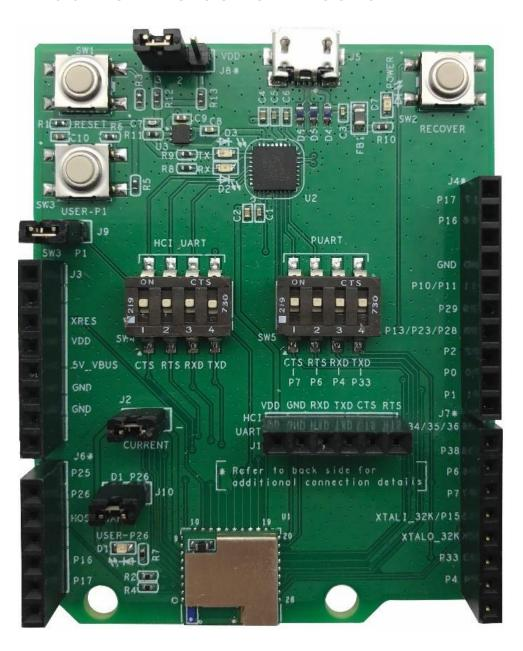
The EZ-BT Module Arduino Evaluation Board (CYBT-423028-EVAL) enables you to evaluate and develop applications on the EZ-BT WICED Module, CYBT-423028-02. CYBT-423028-EVAL can be used as a standalone evaluation kit or can be combined with Arduino compatible shields.
