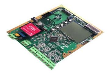
The ATSAM4CMP32-DB demonstration board uses Atmel ATSAM4CMP32C to demonstrate the high accuracy poly-phase energy metering functions. The ATSAM4CMP32C is an integrated poly-phase Energy Metering SoC with 120MHz, dual-core Cortex-M4 ARM processor cores. The board is ETSI format compliant and is designed to interface with CT, Rogowski and Shunt current sensors. The board can interface with ZigBee and PLC communication modules from Atmel.
