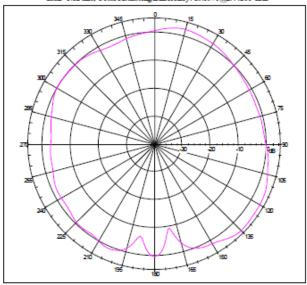
Far-field Power Distribution on Y-Z Plane(H-Plane of L3 Pol Sense) Gain=3.12dBi; Total Radiating Efficiency: 85.65%@2.44200 CHz
