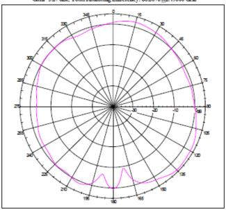
Far-field Power Distribution on Y-Z Plane (H-Plane of L3 Pol Sense) Gain=3.27 dBi; Total Radiating Efficiency: 86.20% @2.45000 GHz
