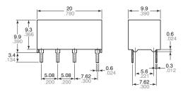
Note: External dimensions of 1 coil latching types are same as single side stable type.
