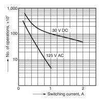
3. Contact reliability for AC loads Tested sample: DS2E-S-DC24V 10 pcs.
