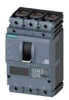
circuit breaker 3VA2 IEC frame 160 breaking capacity class E Icu=200 kA @ 415 V 3-pole motor protection ETU860M, LSIG, In=100A overload protection Ir=40A ... 100A short circuit protection Isd=1,2...15xIn, Ii=3...15xIn cable connection
