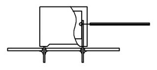
Temperature monitored inside the capacitor.
