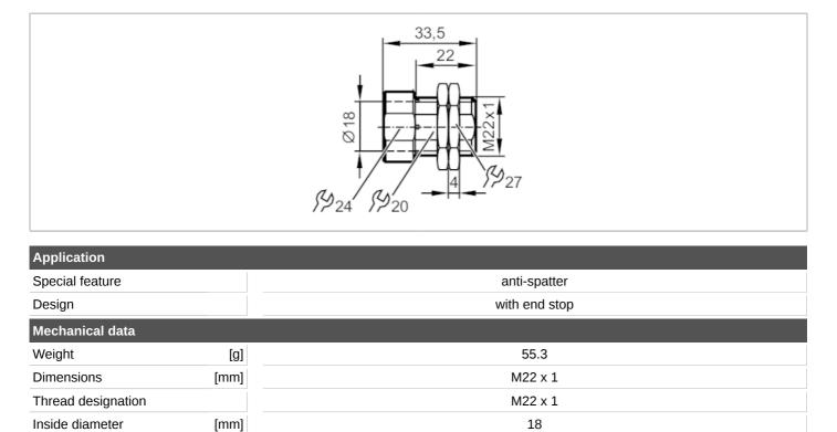
brass anti-spatter; nut: brass anti-spatter
