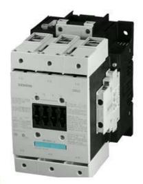
CONTACTOR, 55KW/400V/AC-3 AC(40...60HZ)/DC OPERATION UC 96...127V AUXIL. CONTACTS 2NO+2NC 3-POLE, SIZE S6 WITH BOX TERMINALS ELECTRONIC OPERATING MECHANISM WITH PLC INTERFACE 24V DC SCREW TERMINAL
