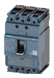
CIRCUIT BREAKER 3VA1 IEC FRAME 160 BREAKING CAPACITY CLASS S ICU=36KA @ 415 V 3-POLE, LINE PROTECTION TM220, ATFM, IN=16A OVERLOAD PROTECTION IR=11,2A ...16A SHORT CIRCUIT PROTECTION II=20 X IN CABLE CONNECTION
