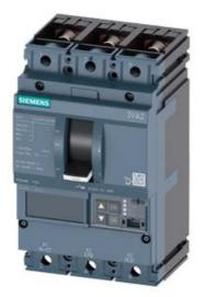
CIRCUIT BREAKER 3VA2 IEC FRAME 100 BREAKING CAPACITY CLASS C ICU=110KA @ 415 V 3POLE, LINE PROTECTION ETU550, LSI, IN=25A OVERLOAD PROTECTION IR=10A ...25A SHORT CIRCUIT PROTECTION ISD=0,6..10X IN, II=1,5..12X IN NEUTRAL PROTECTION OPTIONAL WITH EXT. CT,UPTO 160% BUSBAR CONNECTION
