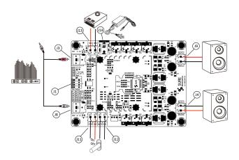
Power Supply Connector: J14 DC Jack 5.5mm/2.5mm J13 Terminal Block RJ128 (optional)
