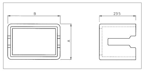
When pins are inserted into the panelmount receptacle half (SMS–R1) of the QIKMATE connector, an optional pin protection shroud can be installed.
