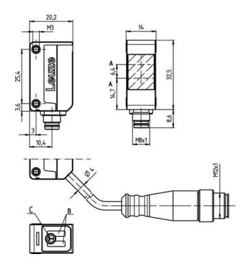
A Optical axis B Indicator diode
