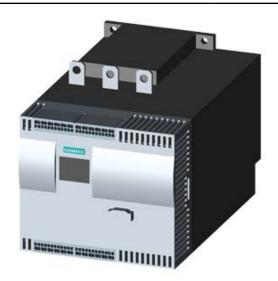
SIRIUS SOFT STARTER, VALUES WITH 575 V, 50 DEG., STANDARD: 117A, 100HP, INSIDE-DELTA CIRCUIT 3: 203A, 200HP, 400-600 V AC, 115 V AC, CAGE CLAMP TERMINALS
