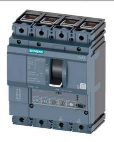
CIRCUIT BREAKER 3VA2 IEC FRAME 160 BREAKING CAPACITY CLASS M ICU=55KA @ 415 V 4POLE, LINE PROTECTION ETU330, LIG, IN=100A OVERLOAD PROTECTION IR=40A ...100A SHORT CIRCUIT PROTECTION II=1,5...12 X IN NEUTRAL PROTECTION ADJUSTABLE(OFF,50%,100%) GROUNDFAULTPROTECTION IG=0,2... 1 X IN, TG=0,1/0,3MS CABLE CONNECTION
