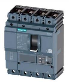
CIRCUIT BREAKER 3VA2 IEC FRAME 160 BREAKING CAPACITY CLASS L ICU=150KA @ 415 V 4POLE, LINE PROTECTION ETU860, LSIG, IN=100A OVERLOAD PROTECTION IR=40A ...100A SHORT CIRCUIT PROTECTION ISD=0,6..10X IN, II=1,5..12X IN NEUTRAL PROTECTION ADJUSTABLE (OFF, UPTO 160%) GROUNDFAULT, SWITCHABLE IG=0,2... 1 X IN, TG=0,050,8MS BUSBAR CONNECTION
