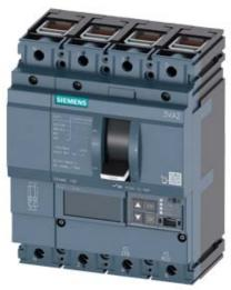
CIRCUIT BREAKER 3VA2 IEC FRAME 160 BREAKING CAPACITY CLASS M ICU=55KA @ 415 V 4POLE, LINE PROTECTION ETU550, LSI, IN=25A OVERLOAD PROTECTION IR=10A ...25A SHORT CIRCUIT PROTECTION ISD=0,6..10X IN, II=1,5..12X IN NEUTRAL PROTECTION ADJUSTABLE (OFF, UPTO 160%) CABLE CONNECTION
