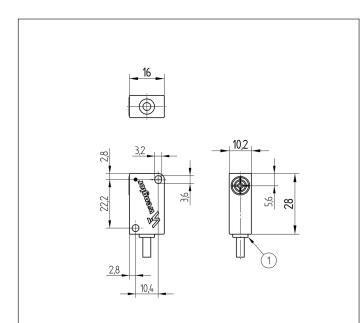
1 = Switching Status Indicator Screw M3 = 0,5 Nm All dimensions in mm (1 mm = 0.03937 Inch)
