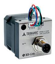
The PD42-1-1243 is a small easy-to-use mechatronic PANdrive™ IO-Link™ actuator device. It combines a NEMA-17 stepper motor with controller and driver electronics. The IO-Link
