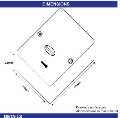
Protection against outside attack. The tactile tamper switch will trigger if the front cover is removed or if the unit is forcibly removed.
