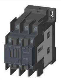
CONTACTOR FOR RAILWAY, AC-3, 18.5KW/400V, 1NO+1NC, . DC 24V, 0.7...1.25\*US, W. VARISTOR INTEGRATED, 3POLE SZ. S0, RING CABLE LUG CONNECTION
