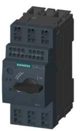
CIRCUIT-BREAKER SZ S00, FOR MOTOR PROTECTION, CLASS 10, A-REL. 0.35...0.5A,N-RELEASE 6.5A SPRING-L. CONNECTION STANDARD SW. CAPACITY W. TRANSVERSE AUX. SWITCH 1NO+1NC
