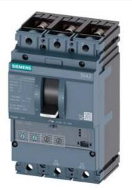
CIRCUIT BREAKER 3VA2 IEC FRAME 100 BREAKING CAPACITY CLASS C ICU=110KA @ 415 V 3POLE, LINE PROTECTION ETU350, LSI, IN=40A OVERLOAD PROTECTION IR=16A ...40A SHORT CIRCUIT PROTECTION ISD=1,5... 10 X IR, II=12 X IN BUSBAR CONNECTION
