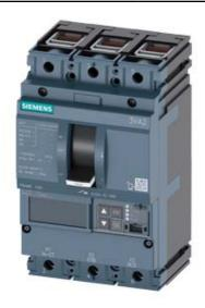
CIRCUIT BREAKER 3VA2 IEC FRAME 160 BREAKING CAPACITY CLASS M ICU=55KA @ 415 V 3POLE, LINE PROTECTION ETU860, LSIG, IN=40A OVERLOAD PROTECTION IR=16A ...40A SHORT CIRCUIT PROTECTION ISD=0,6..10X IN, II=1,5...12X IN NEUTRAL PROTECTION OPTIONAL WITH EXT. CT,UPTO 160% GROUNDFAULT, SWITCHABLE IG=0,2... 1 X IN, TG=0,050,8MS CABLE CONNECTION
