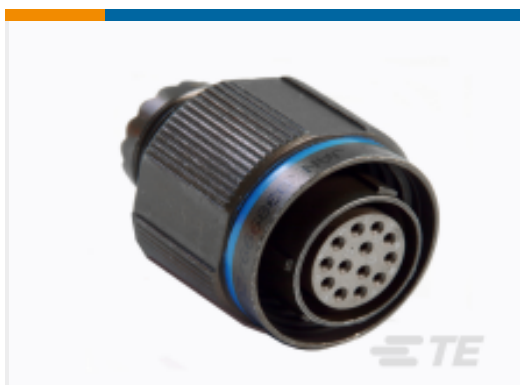
TE Part #YDTS26F13-04SEV001 Straight Plug: D38999, 13-04 Insert, Electroless Nickel Plating
