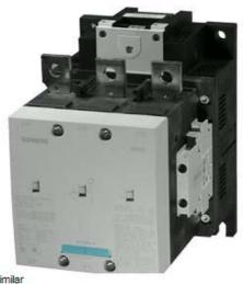
VAC. CONTACTOR, 110KW/400V/AC-3 AC(40...60HZ)/DC OPERATION UC 21-27.3V AUXILIARY CONTACTS 2NO+2NC 3-POLE, SIZE S10 BAR CONNECTIONS ELECTRONIC OPERATING MECHANISM WITH 24V DC PLC INTERFACE
