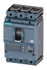
CIRCUIT BREAKER 3VA2 IEC FRAME 160 BREAKING CAPACITY CLASS C ICU=110KA @ 415 V 3POLE, LINE PROTECTION ETU560, LSIG, IN=63A OVERLOAD PROTECTION IR=25A ...63A SHORT CIRCUIT PROTECTION ISD=0,6..10X IN, II=1,5..12X IN NEUTRAL PROTECTION OPTIONAL WITH EXT. CT,UPTO 160% GROUNDFAULT, SWITCHABLE IG=0,2... 1 X IN, TG=0,050,8MS CABLE CONNECTION
