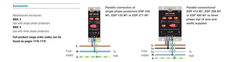
**NOTE:** If you desire a protector with an extra high maximum surge current use the ESP M2 or ESP M4 series. If your supply is fused at 32 amps, or less, the in-line protectors (ESP 240 or 120-5A (or -16A) and their ready-boxed derivatives, or ESP D/DS 10 or 32A Series) may be more suitable. If you need to mount the display panel separately from the main protector unit, use the ESP M1R series.
