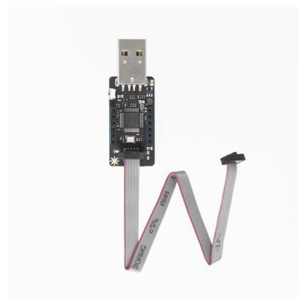
The Particle Debugger gives you the power of professional debugging at a fraction of the cost. Using this accessory, you'll be able to program Particle mesh-ready hardware over common interfaces like JTAG and SWD, using open source tools like GDB.
