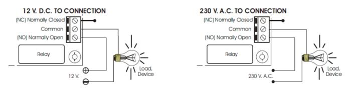
**CONSIDERATION TO THE OUTPUT. LOAD.** During to the operating the module according to be charge, you can happen the fluctuation or incorrect output functionament. This is wrong you have install the anti-spark (resistor & capacitor), between two contacts of the relay make's in the connection such as is to apper in the
