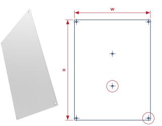
Mounting plates are supplied with 1-3 central fixing holes depending on size for additional anchoring and stability against sagging when installing heavier components.
