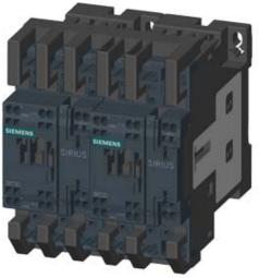
REV. COMB., AC3, 15KW/400V DC24V 3-POLE, SZ S0 SPRING-LOADED TERMINAL ELECTR. AND MECH. INTERLOCK 2NO INTEGR.
