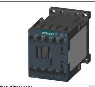
CONTACTOR, AC-3, 7.5KW/400V, 1NC, DC 48V, 3-POLE, SZ S00 SCREW TERMINAL
